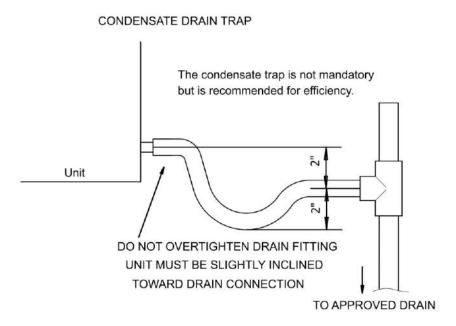
Figure 4-2 Condensate drain trap
