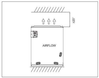
Figure 3-1 Clearance requirements
