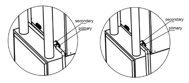
Figure 4-1 Drain connections
