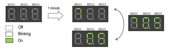
**Refrigerant coefficient** is used to evaluate the refrigerant level in the ecoer systems.
