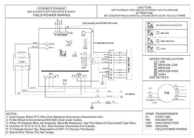
Figure 4-1 Wiring Diagram
