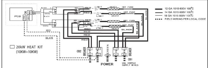
Figure 4-3 Wiring diagram for electric heat
