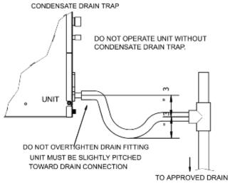
Figure 7-1 Condensate drain trap
