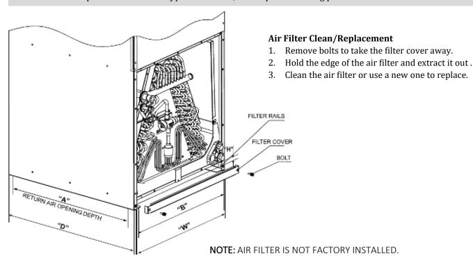
Figure 8-1 Filter installation and clean
