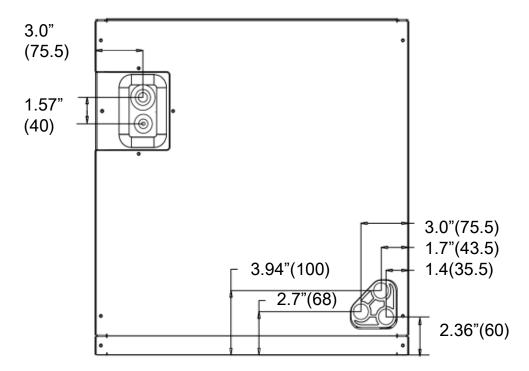
Figure 3-1 Dimensions for front connection coil
