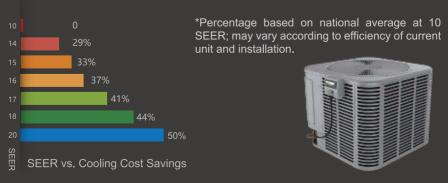
Ecoer Inverter systems deliver the precise amount of heating and cooling needed to achieve the desired temperature, no more/no less. Thanks to a SEER rating up to 20, a HSPF rating up to 10 and a self-learning load programming, the inverter system can reduce annual utility bills up to 50% compared to older 10 SEER systems. Ecoer systems provide the greatest indoor comfort at the most affordable price to our customers.
