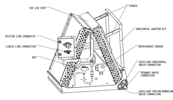
Figure 3-2 Indoor coil and drain pan set-up
