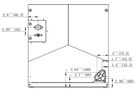
Figure 3-1 Dimensions for front connection coil
