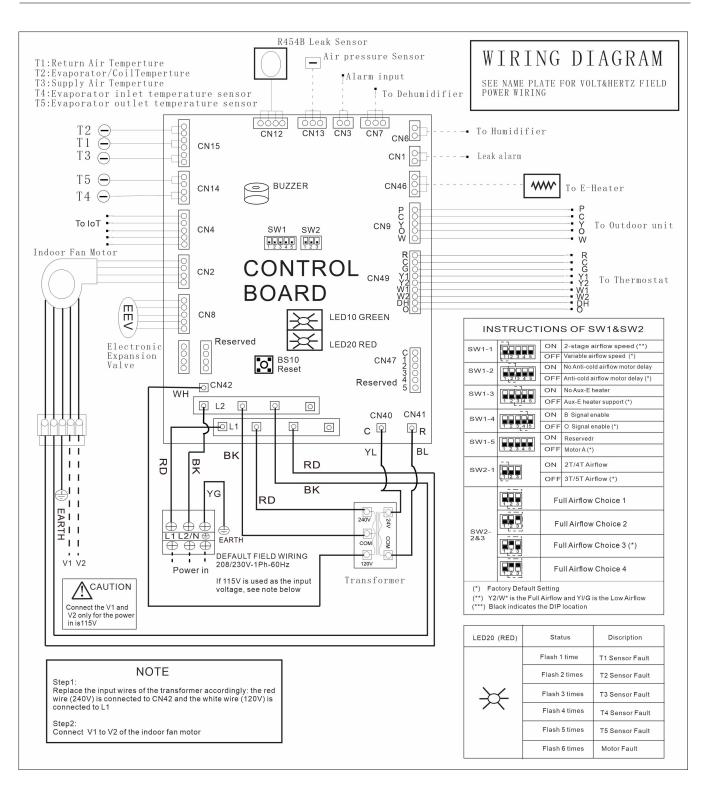
Figure 4-1 Indoor unit Wiring Diagram
