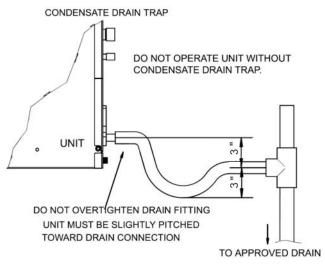
Figure 7-1 Condensate drain trap
