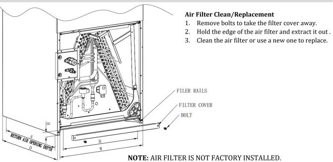
Figure 8-1 Filter installation and clean
