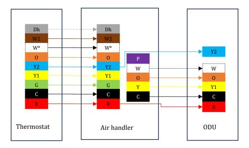
• Wiring for 2H1C thermostat (setting 2-stage airflow)
