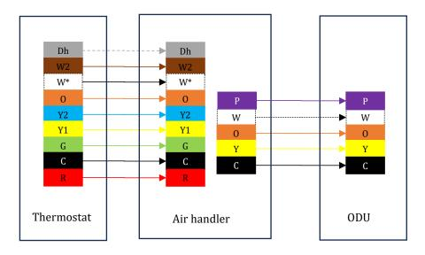
• Wiring for 2H1C thermostat (support auto airflow)
