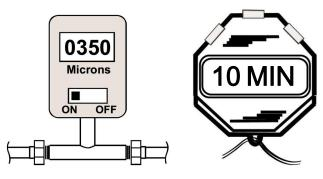
Fig 8-1 Evacuation the refrigerant system
