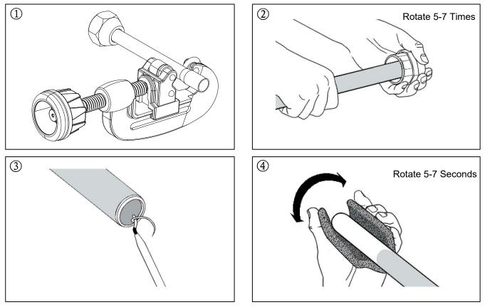
Fig 6-2 Refrigerant Line Press Fitting Connection
