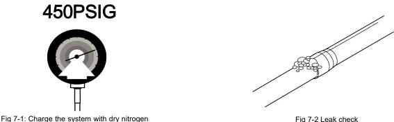
After completion of field piping for split systems, the field pipework shall be pressure tested with nitrogen and then vacuum tested prior to refrigerant charging, according to the following requirements:
