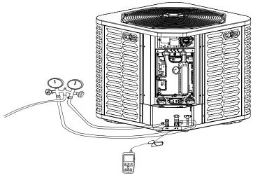
Fig 13-3 Measure the superheat or sub-cooling
