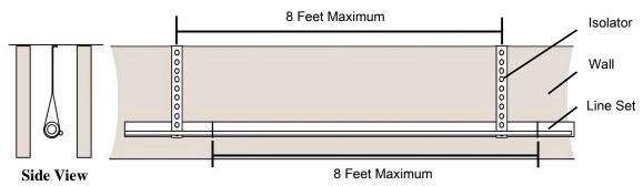
Secure suction line using isolators every 8 ft. Secure liquid line directly to insulated suction line using tape, wire, or other appropriate method every 8 ft.
