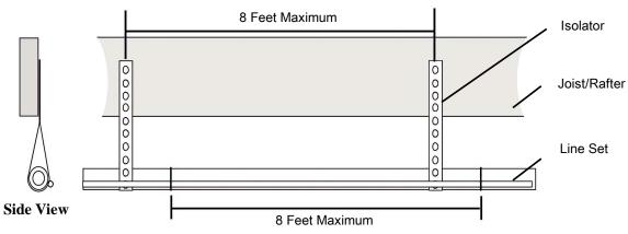
Secure suction line from joists using isolators every 8 ft. Secure liquid line directly to insulated suction line using tape, wire, or other appropriate method every 8 ft.
