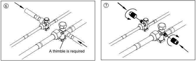
Fig 6-1 Refrigerant Line Brazing Connection
