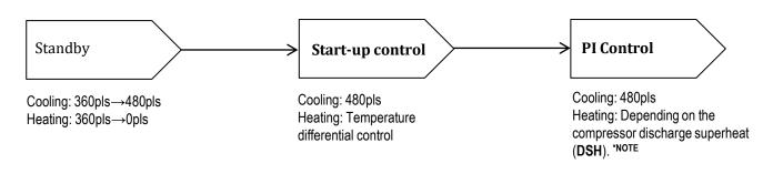
NOTE: Heating DSH should be between 25°F and 60°F with proper refrigerant level.
