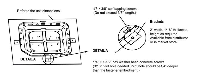
Fig 3-2 Fasten the condensing unit
